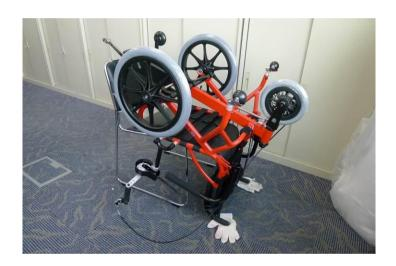
Turn Profhand upside down, and place it onto the working platform, have the push handles rest on the floor, make sure to place soft materials to act as shock absorbers, to refrain from damaging it, also make sure that the control lever doesn't make contact with the floor are platform.
